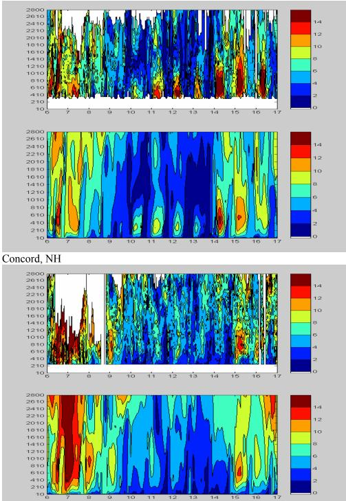
Figure 4: MM5 and Wind profiler comparison for August 6 to 17, 2002 at Richmond, VA and Concord, NH. The upper and lower panes at each station are for MM5 and profiler, respectively. The abcissa represents day and the ordinate the height (m).
