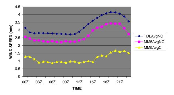
Figure 7: Comparison of averaged wind speed between MM5 and observed under calm (C) and non-calm (NC) conditions.
