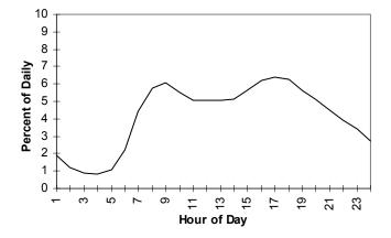
Using the I-80 segment for 1990, typical hourly volumes which result include:8-9 a.m. $6.0\% \times (41,111 \text{ vehicle miles}/ 0.296\text{mi.}) = 833 \text{ vehicles/hour (vph)}$ 12-1 p.m. $5.0\% \times (41,111 \text{ vehicle .miles}/ 0.296\text{mi.}) = 694 \text{ vph}$ 5-6 p.m. $6.3\% \times (41,111 \text{ vehicle miles}/ 0.296\text{mi.}) = 875 \text{ vph}$
