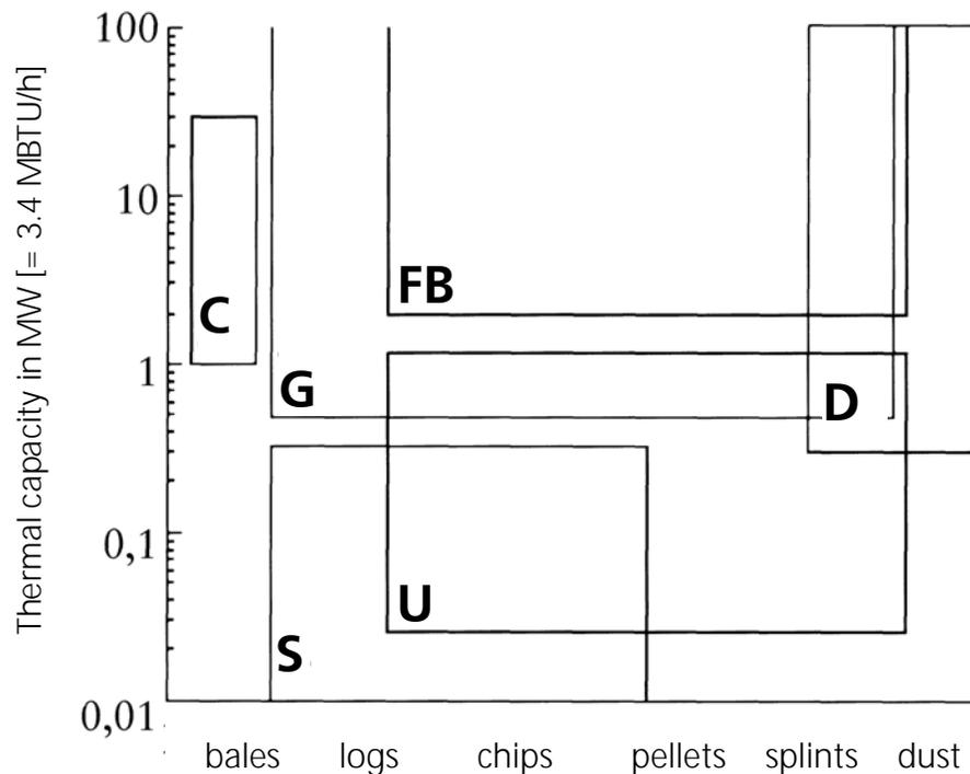
( C Cigar burner, G Grate firing, S Shaft firing, U Underfed Stoker, FB Fluidized Bed, D Dust suspension firing)
