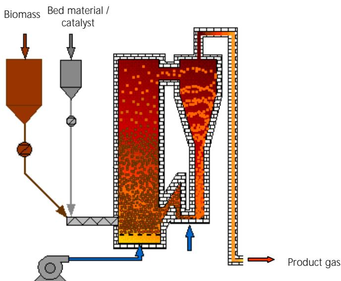
The drawback of fluidized bed gasification is the increased particulate loading in the produced gas, which is about one magnitude higher compared to fixed bed reactors. Therefore, dust removal from the produced gas is essential.
