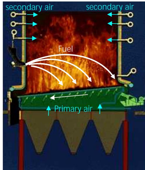
In general, grate firing combustors are able to burn a variety of fuels, but the fuel has to be very well mixed and have a constant moisture content. Otherwise grate areas with incomplete ignition / combustion may occur. The upwards-moving gases of these areas contain high amounts of carbon monoxide (CO) and volatile
