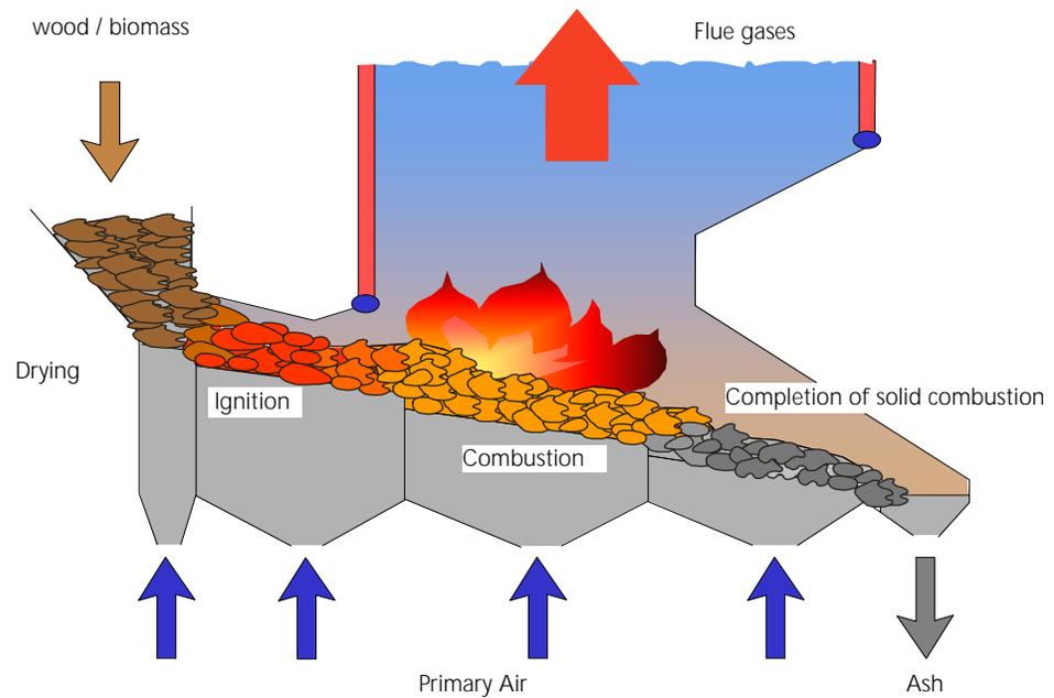
As the fuel travels on the grate, it passes the drying, ignition, combustion and the burnout zone. Primary air is supplied from the bottom through the grate. Secondary Air is supplied from above to complete the combustion of the gases.
