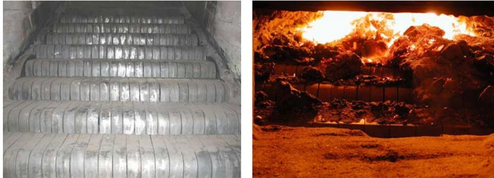
One special type of grate combustor is the spreader stoker (Figure 3-11), in which the wood is catapulted from one side above the grate. Small particles already combust during flight. Large, heavy particles cover the greatest horizontal distance before they drop onto the grate. Due to the fact that the grate transports the fuel layer back towards the side of the fuel supply, large fuel pieces have the longest residence time in the combustion zone.
