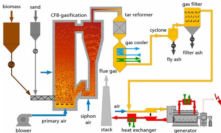
The catalyst is operating at the high temperature of the gas leaving the gasifier. If a CFB gasifier is used, the catalyst has to be able to handle the high dust content of the hot gas. Therefore, preferred technologies are based on monolith catalysts in a honeycomb design or fluidized catalytic beds. Even though the fluidization velocity of such fluidized bed catalytic systems is much lower than the gas velocities in fluidized bed gasifiers, entrainment of the catalyst still presents a problem.
