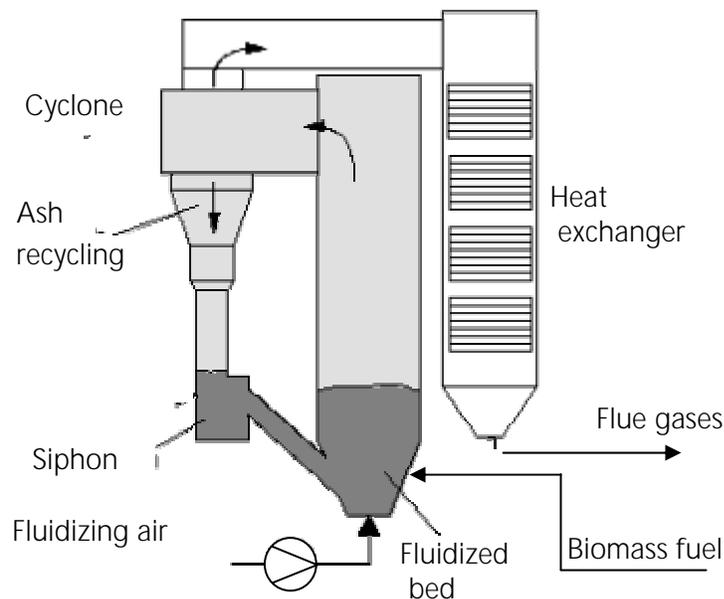
In fluidized bed combustion systems, the heat is extracted from the bubbling bed by using submerged heat exchange surfaces (tube bundles) or water-cooled walls. Circulating fluidized bed systems also use the reactor walls as heat exchange surfaces and, sometimes, additional heat exchangers. These add-on heat exchangers are partially submerged into the bed below the cyclone.
