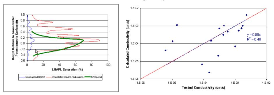
Figure 6 Comparison of Tested Versus Calculated NAPL Conductivities
