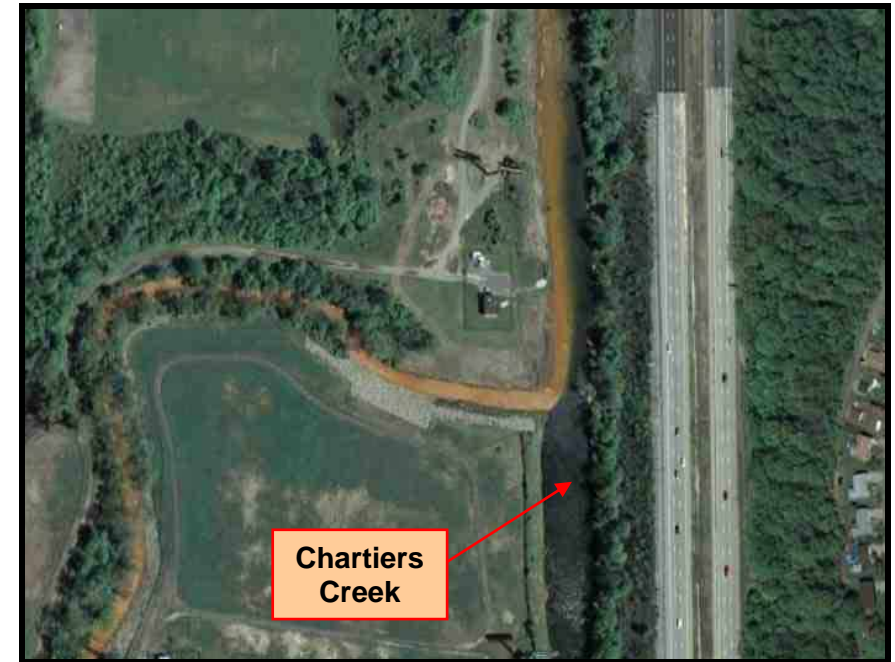
Figure 3 – Gladden discharge and weir (upper left), Gladden Discharge entering Millers Run (upper right), Millers Run below the Gladden Discharge (lower left), and an aerial view of the confluence of Millers Run and Chartiers Creek showing iron plume (lower right).
