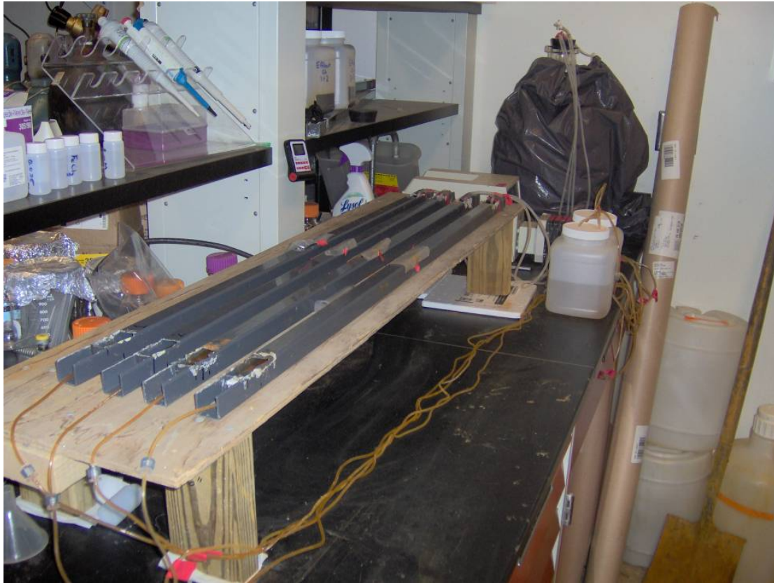
Figure 2. Photos of “gutter” reactors constructed and operated in the Environmental Engineering Laboratories at Penn State University. Water flows from the upper right to the lower left through square PVC tubes (1-in square by 36-in long). A large carboy filled with Hughes Borehole water is wrapped in brown plastic to exclude light and is continuously purged with N 2 (g) to minimize Fe(II) oxidation during storage and use. A peristaltic pump (barely visible behind the upper end of the reactors) is used to convey water from the carboy to the top of the gutters. Two of the gutters were filled with approximately 125 g of sediment, packed to a sediment bed thickness of ca. 0.25 in, while the other two gutters contained no sediment.
