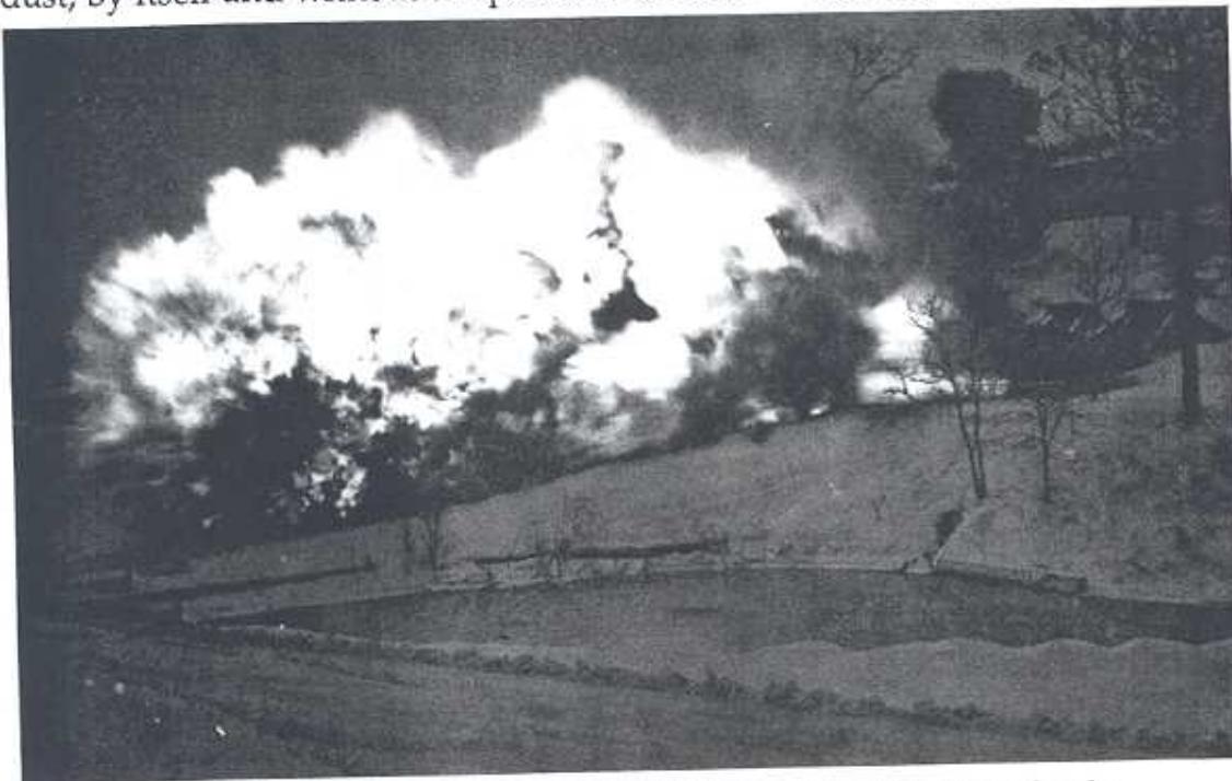
Coal dust explosion from main entry, Experimental Mine, Bruceton, Pennsylvania.
