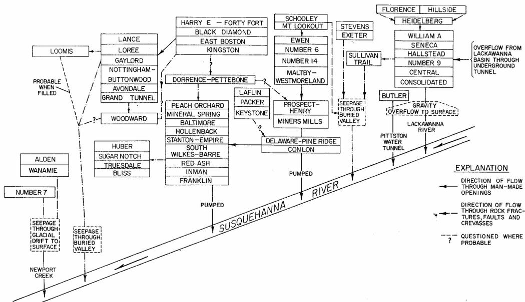
**Figure 2.14.** Schematic diagram of water flow through the mines (eg. Barrier pillar breaches) in the Wyoming Basin, (from Hollowell 1971).
