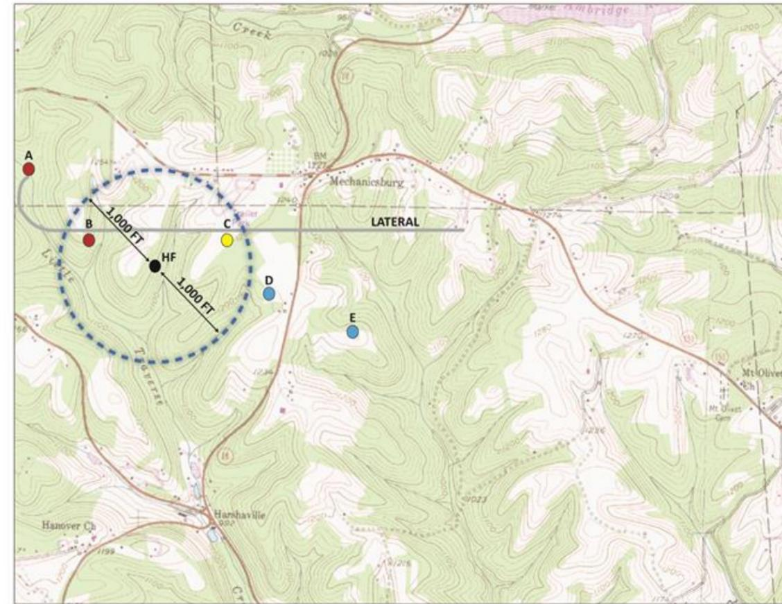
Notes: Yellow (identify); Red (identify and visually monitor); and Blue (no requirements); HF (well that is subject of area of review that will be hydraulically fractured)
