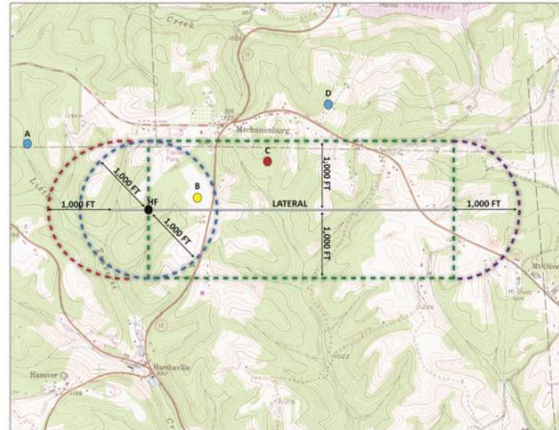
Notes: Yellow (identify); Red (identify and visually monitor); and Blue (no requirements); HF (well that is subject of area of review that will be hydraulically fractured); geometry depicted is similar to that for a *deep conventional well* (oil or gas) that has been intentionally deviated
