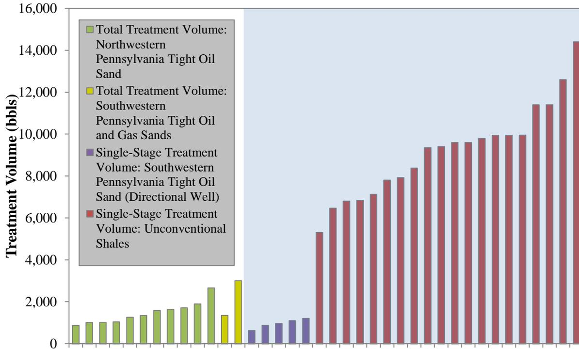
Figure B. Graphical summary of total and single-stage treatment volumes gathered as part of the *hydraulic fracturing* study. Blue-shaded portion of diagram highlights directional completions in Upper Devonian tight sands, the Marcellus shale, and the Utica shale.
