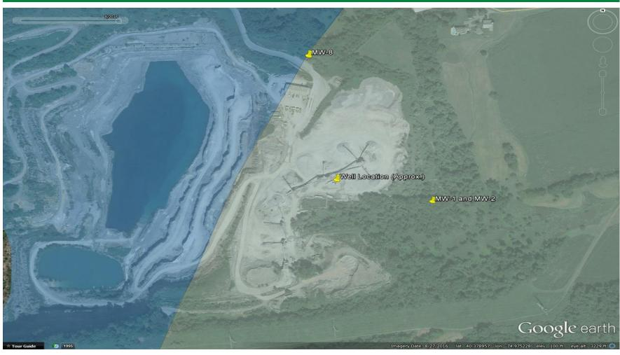
Monitoring well locations are noted by MW1 and MW2 to the right and MW8 at the top center. The fourth in the center is for the plants water use.
