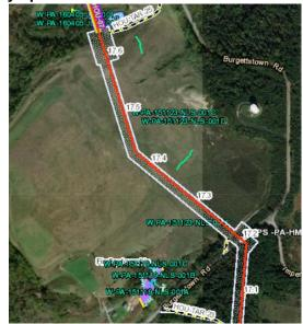
The Project does cross a coal refuse pile from approximately MP15.85 to 16.2 via HDD HOU-06. The actual refuse pile will not be disturbed because the HDD will cross below the pile; therefore, no additional permits are required. If a coal refuse pile is discovered during construction, the construction crews evaluate the situation and determine the best course of action. No refuse material will be placed back into the trench to be used as fill.
