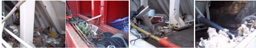
Figure 2-1 Examples of Materials Behind Rear Load Truck Ejection Blades
