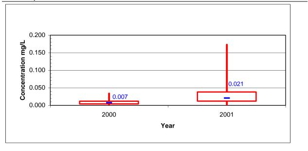
Figure 9. Comparison of HAA5 results of the 23 retested small surface water filtration plants. The line in the center of the box and nearby number is the median value of each filtration plant.
