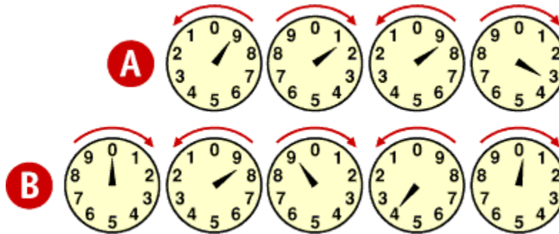
Figure 3.1 An Electric Meter 1
