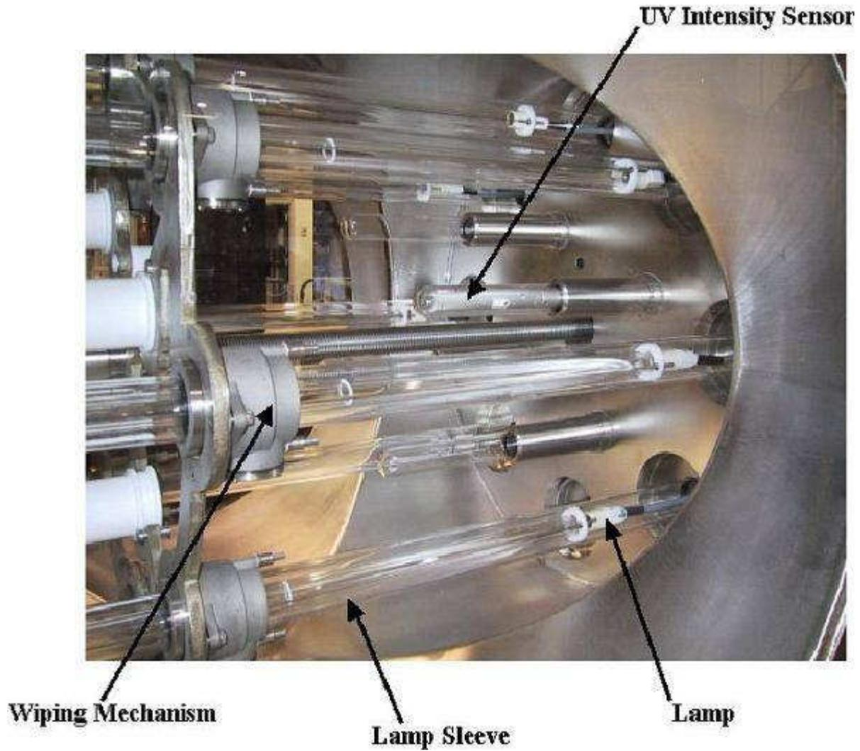
Figure 2.3 The Inside of a Reactor<sup>3</sup>
