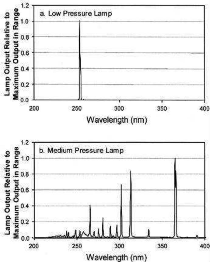
Figure 2.5 – UV Lamp Output: LP vs. MP<sup>5</sup>
