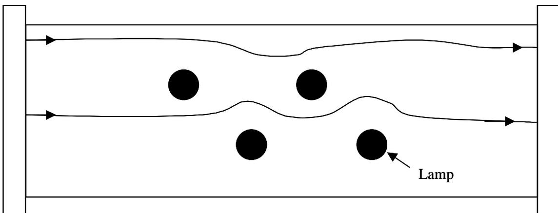
Figure 3.1 Reactor with Lamps.
