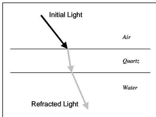
Figure 1.4 – Refraction
