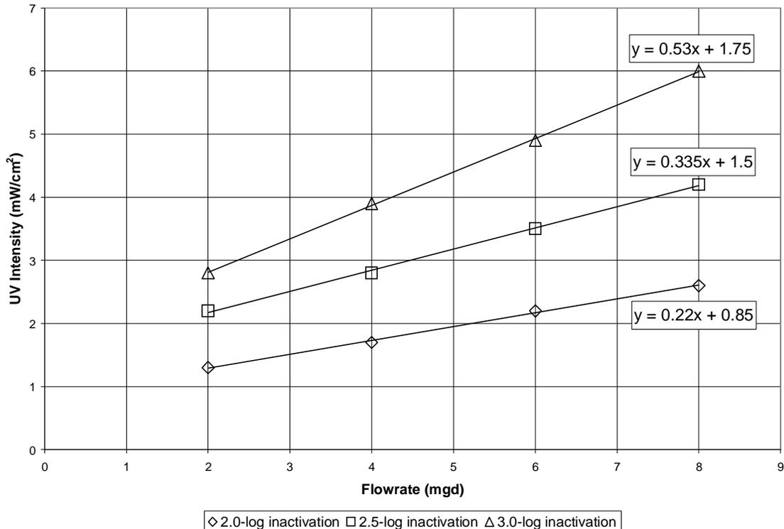
Figure 4.1 – UV Intensity Setpoint Interpolation Graph
