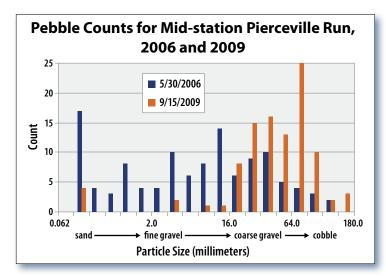
Figure 2. Pre- and post-project pebble counts for Pierceville Run show a trend toward coarser gravel and cobbles, an indication of improving conditions.
