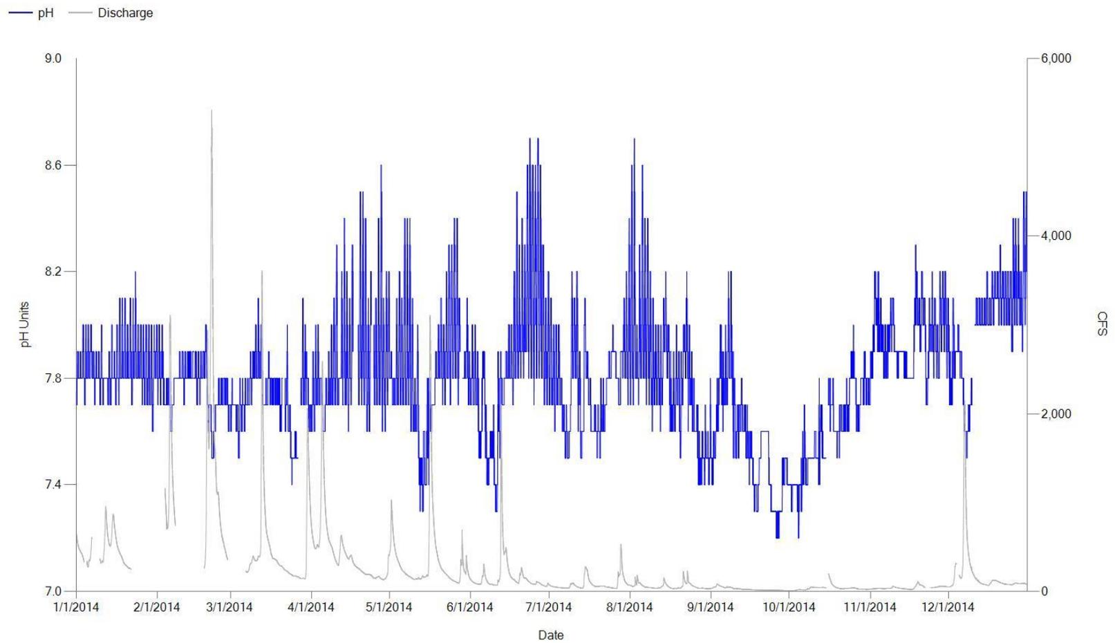
Figure 7. Continuous pH measurements from January 1, 2014 to December 31, 2014 showing the response to elevated discharge events.
