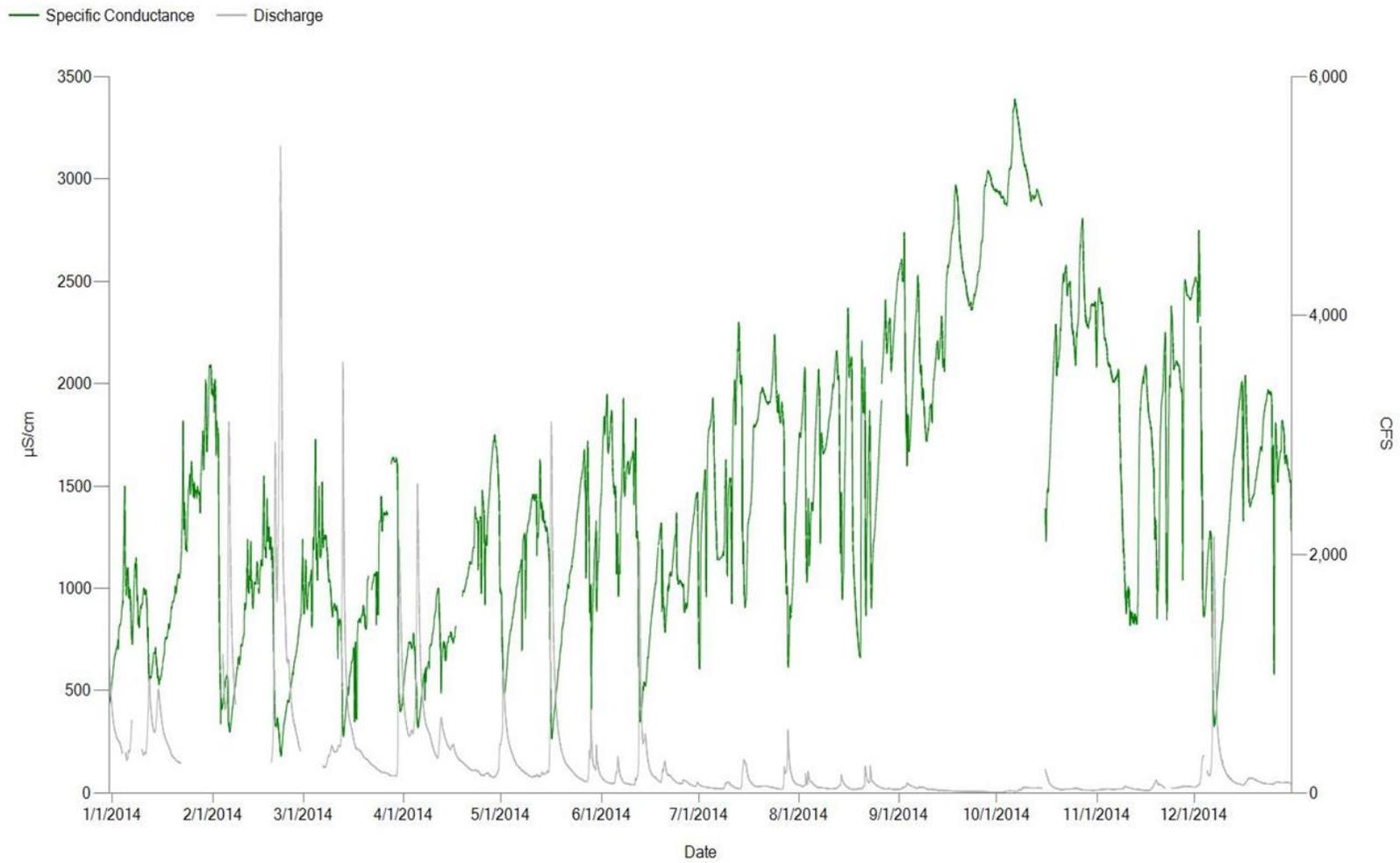
Figure 5. Continuous specific conductance from January 1, 2014 to December 31, 2014 illustrating depressed readings in response to elevated discharge events.
