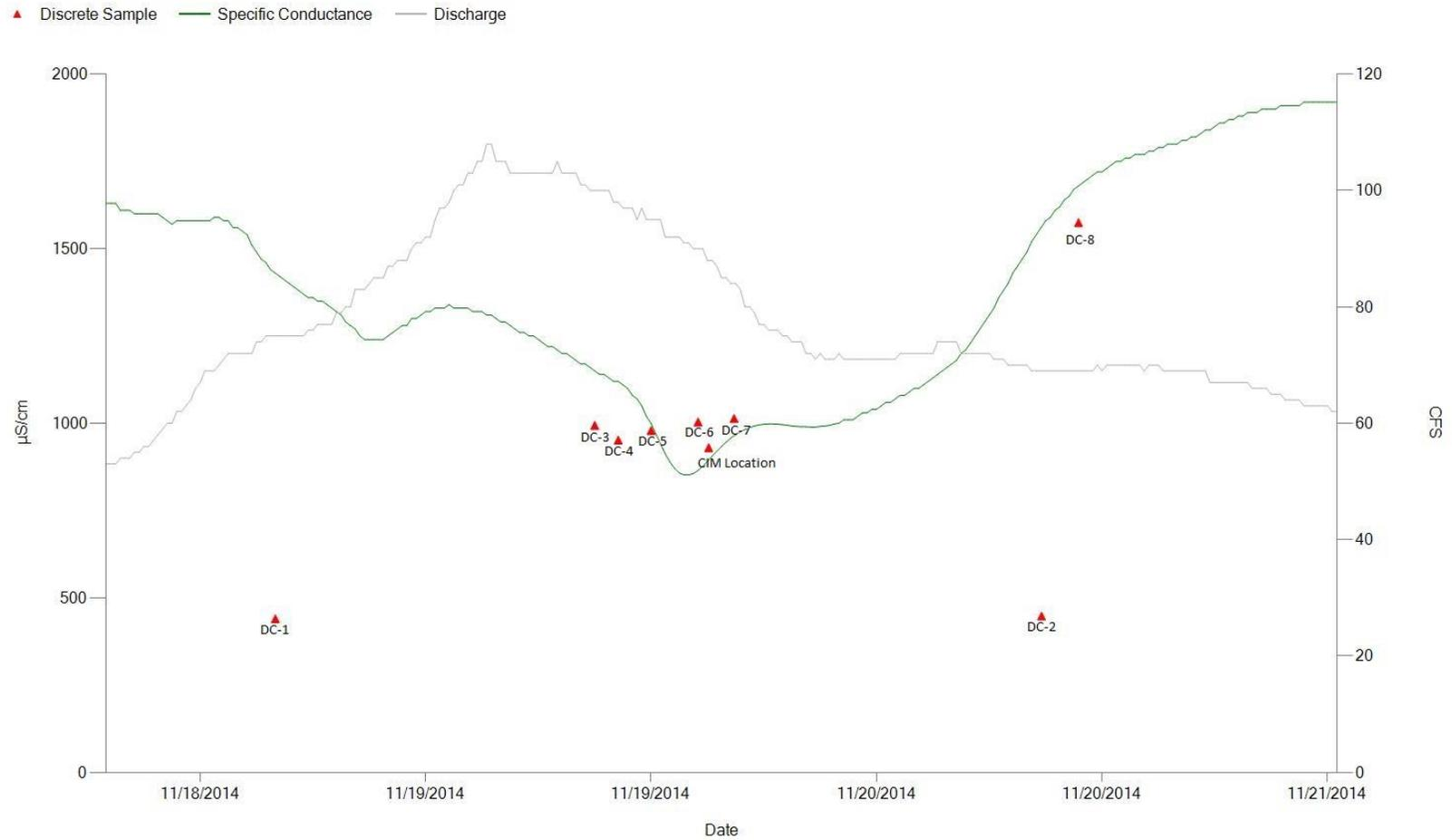
Figure 10. Specific conductance CIM data overlaid by discrete water quality readings taken during the stream assessment field data collection from November 18 to November 20, 2014.
