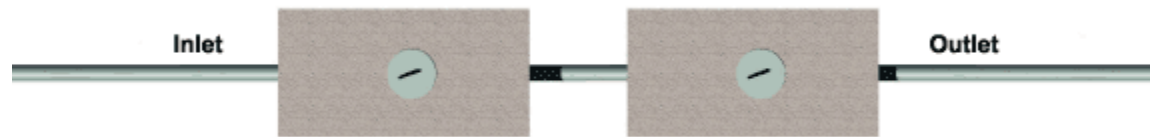
Rectangular Septic Tanks in Series
