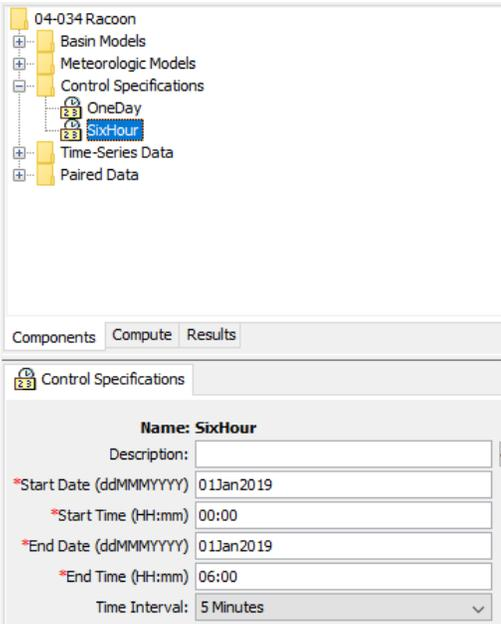
The HEC-HMS model should be used to compute the conditions at the dam for all five of the distributions. These results should be compared. The PMF for the dam is the flood that results in the highest peak outflow and the maximum water surface elevation in the impoundment. The following spreadsheet shows these results at the sample dam, where the Storm Specific 3HR is designated as the PMF because it has the highest outflow and maximum water surface elevation.
