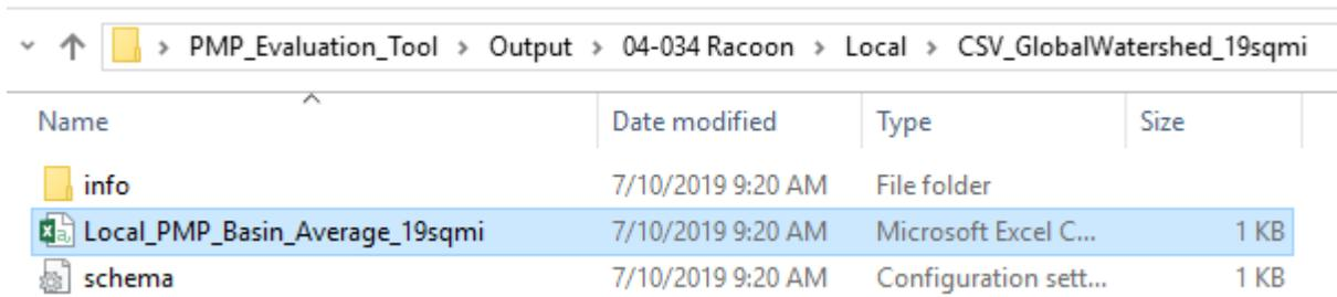
The spreadsheet highlighted above (Local\_PMP\_Basin\_Average\_19sqmi) when opened (see below) provides the Local Storm PMP rainfall depths for 1 through 24 hour durations. The rainfall depths to be copied into the PMP tool are designated by the red arrows.
