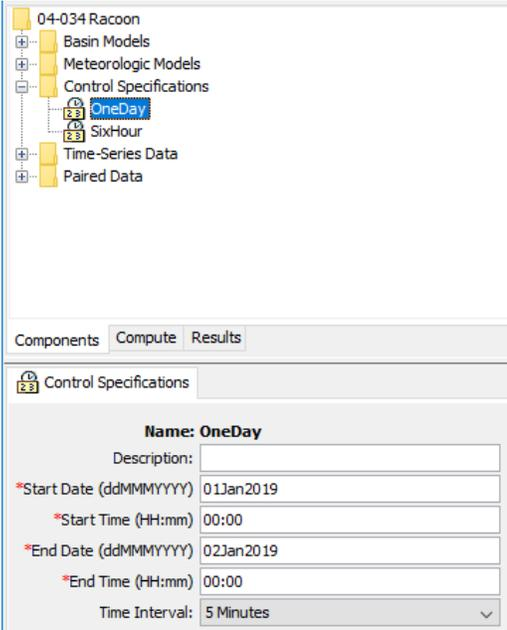
**2-hour Synthetic 6-hour control specification:**
