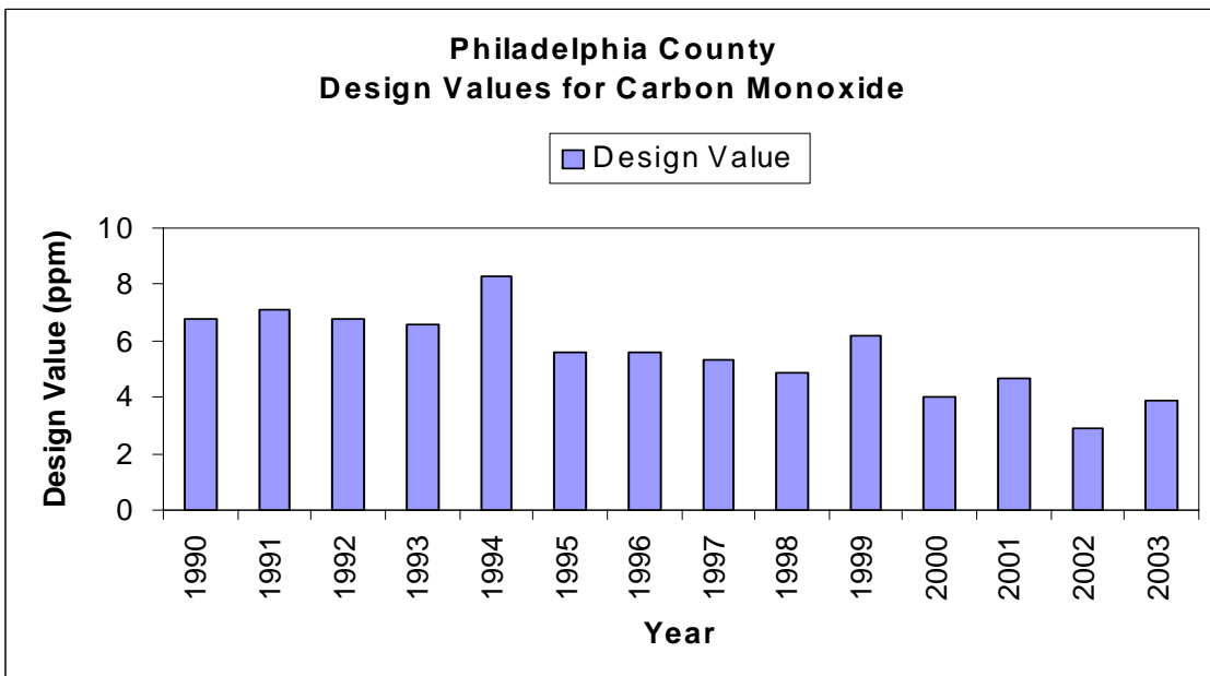
Figure 2 - Philadelphia County Design Values for Carbon Monoxide - Time Versus CO Concentration From 1990 Through 2003
