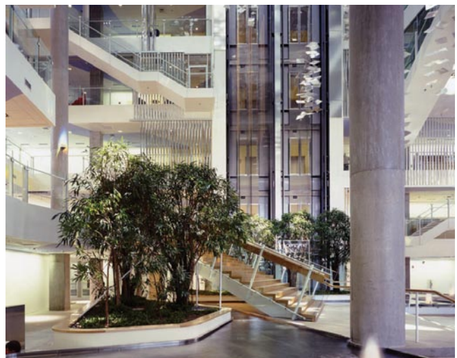
Genzyme, a biotechnology company, designed its corporate headquarters in Cambridge, MA to be extremely energy-efficient, with electricity costs about 42 percent less than a comparable building. Use of daylight allows 75 percent of employees to work with natural light alone. 17
