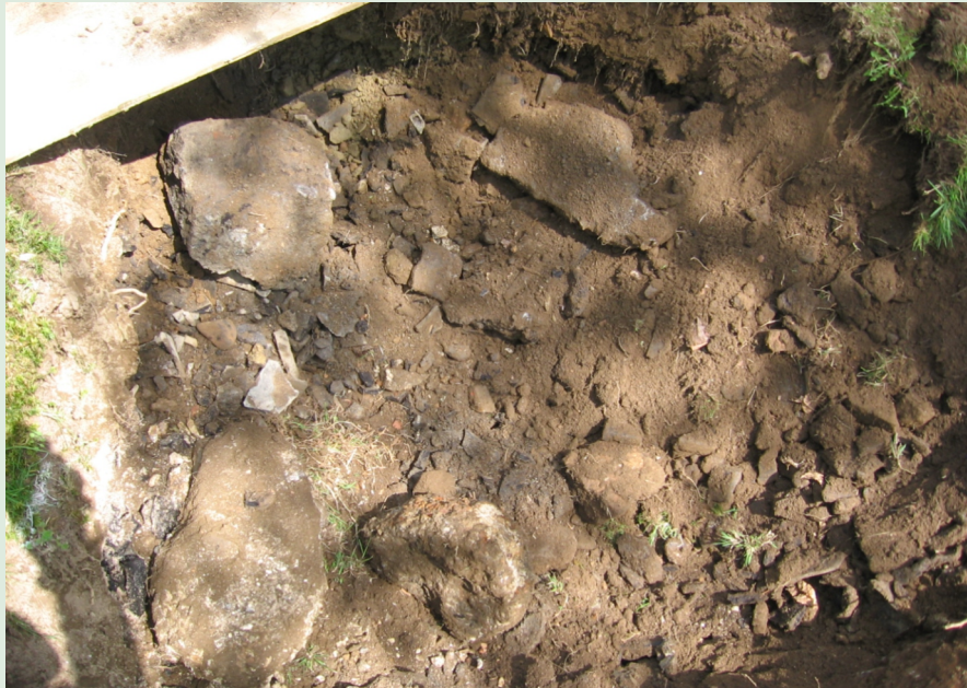
Battery casing material intermingled with soil, cobbles and other fill material that was used pre-1990 to raise and level residential yards at the Mt. Laurel Battery Casing Site, Alsace Township, Berks County, Pennsylvania.
