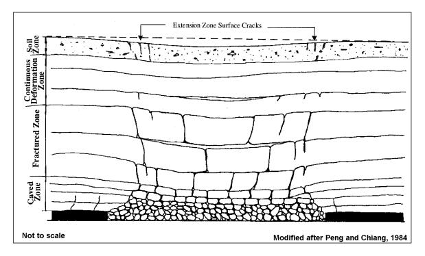
Figure VIII.2 Overburden Movement above a Longwall Panel
