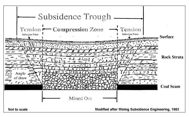
Ground movements within a subsidence trough have both vertical and horizontal components. Downward vertical movement usually occurs at all areas within the trough. The vertical movement is usually greatest at the center, and it progressively decreases at points along the trough profile until the limit of the affected surface area is reached. The Department's investigators have also observed instances where slight "heave" or upward movement has occurred.
