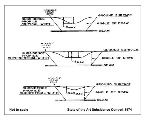
Figure VIII.4 Critical, Supercritical, and Subcritical Widths
