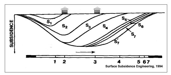
Figure VIII.5 Development of Dynamic Subsidence Profiles as the Face Advances
