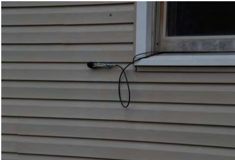
Figure 1.5 Airblast microphone located outside the House.
