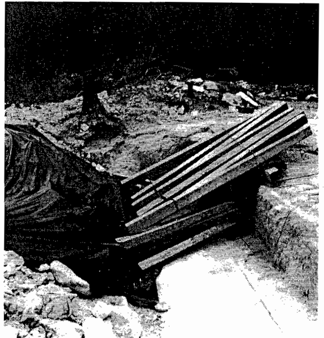
FIGURE 4.—Pit area with blasting mat and timbers covering test shot.
