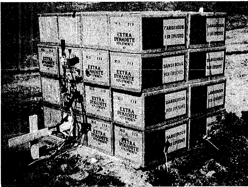
FIGURE 9. - Dynamite Acceptor Showing Instrumentation and D'Auric Leads.
