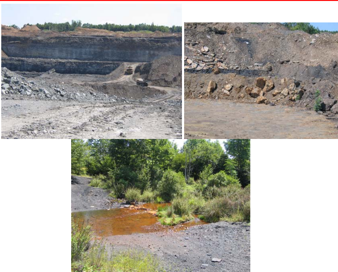
Figure 6. The Kasubic Operation showing the principal pit, and a pit where the Johnstown Limestone is obtained for alkaline redistribution throughout the mine. The lighter colored, irregular-shaped blocks are limestone. XL monitoring point is on Morgan Run, above.
