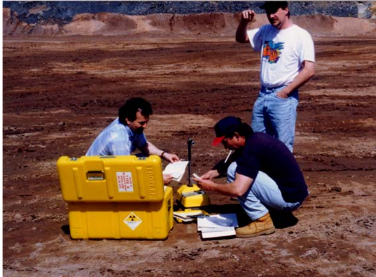
Figure 9.6. Mike Menghini, Tom Owen, and Mike Wehr using Troxler nuclear density moisture gauge on the lower ash terrace.
