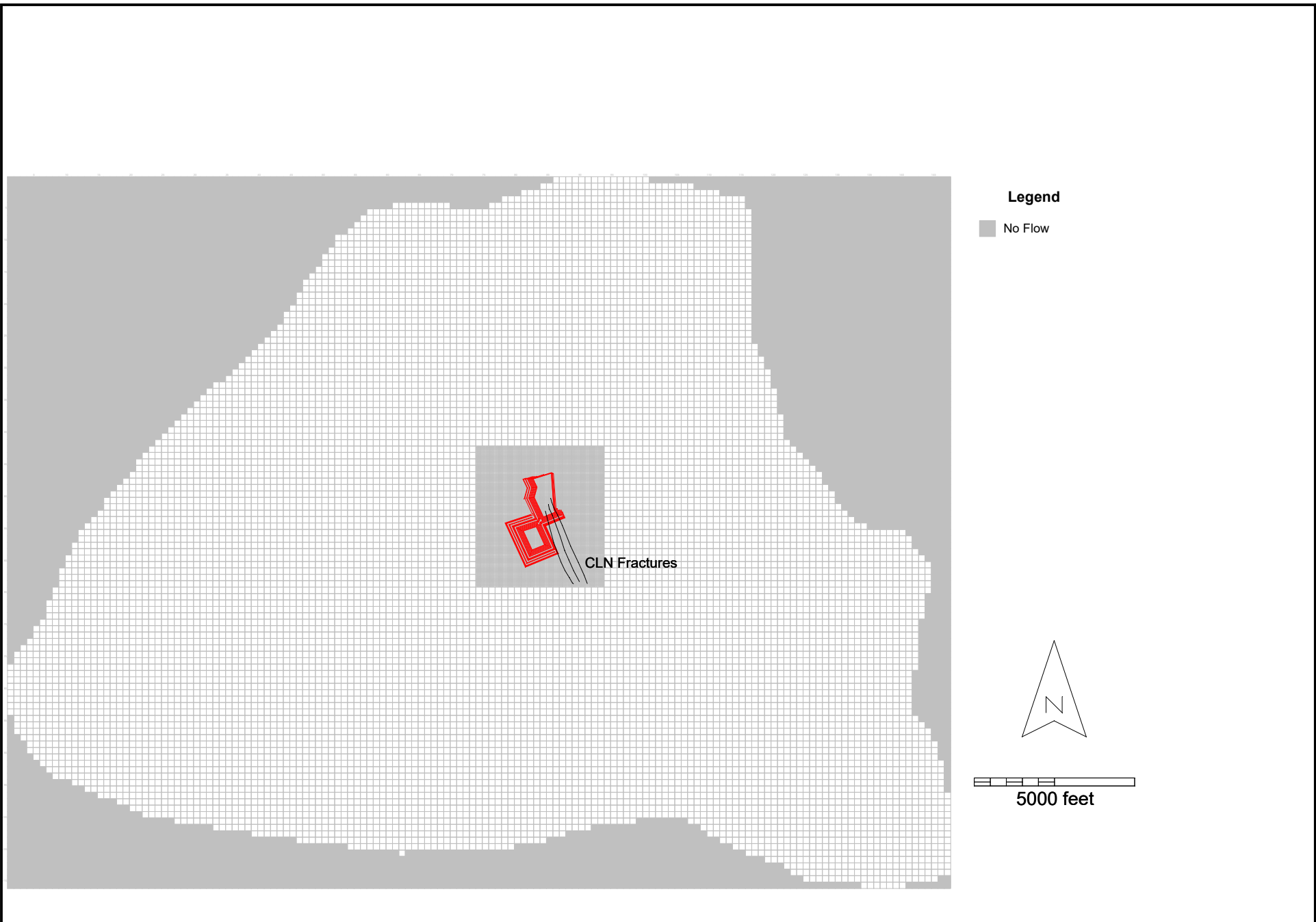
Figure 2-1 Model Grid for the Pierson Rheems Groundwater Model.
