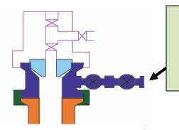
Section 13: Primary Production Gas Pressure (measured inside primary production casing)
