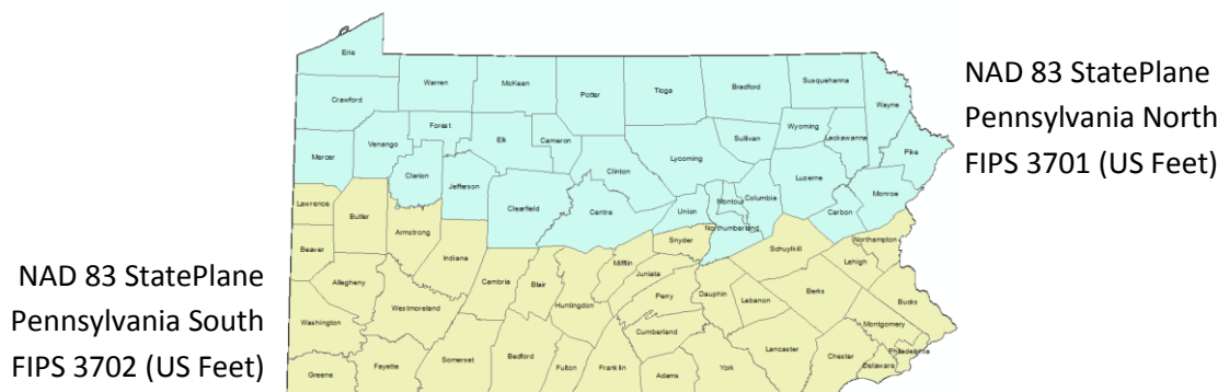
Figure 1: Shows a map of the two State Plane Coordinate System zones, showing the counties that make up each zone.
