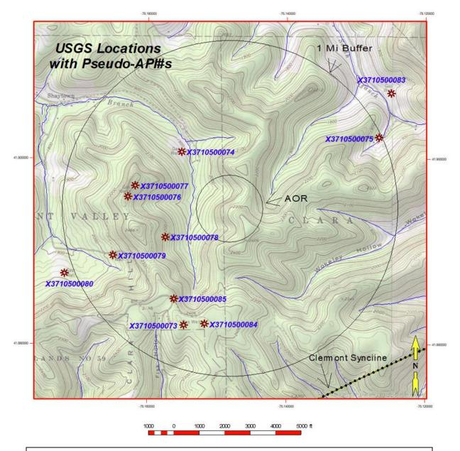
There are nine (9) locations within the 1 mile buffer that were annotated by the USGS on the Shinglehouse 7.5 minute topographic quadrangle map. These locations are not part of the DEP/DCNR databases and therefore are given pseudo-API #s to differentiate them from wells within the State databases.
