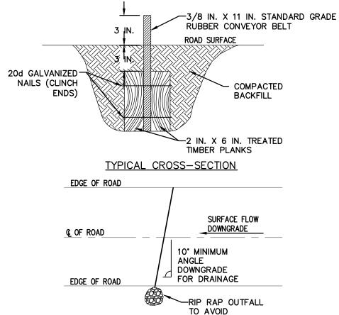
1. DEFLECTORS SHALL BE USED ON TEMPORARY ACCESS ROADS WITH SLOPES GREATER THAN 10 PERCENT. MAXIMUM DEFLECTOR SPACING SHALL BE 100 FEET.
