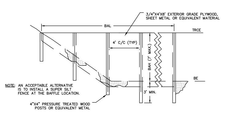
IN POOLS WITH DEPTHS EXCEEDING 7', THE TOP OF THE PLYWOOD BAFFLE DOES NOT NEED TO EXTEND TO THE TEMPORARY RISER CREST. SUPER SILT FENCE BAFFLES NEED NOT EXTEND TO TRCE ELEVATION.
