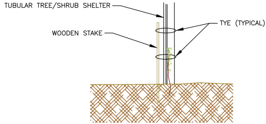
NOTE: TREE/SHRUB SHELTERS ARE TO BE MADE FROM BIODEGRADABLE PLASTIC TUBING. SIZE OF SHELTERS AND WOODEN STAKE TO BE DETERMINED BY PROJECT MANAGER.
