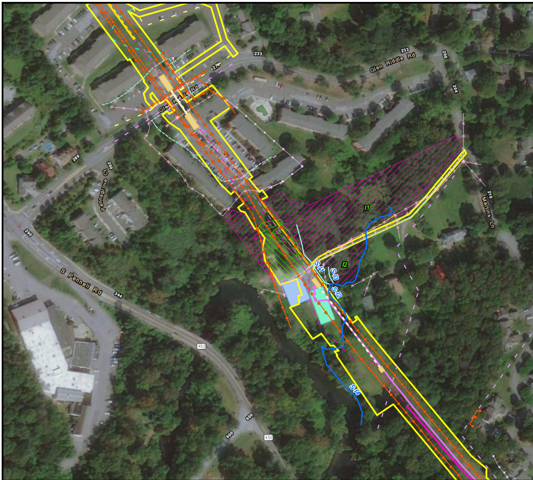
Figure 1. Aboveground and Buried Utility Infrastructure Constraints in the Vicinity of Aquatic Resource Crossings. Proposed 0620 HDD Installation Method Change, Middletown Township, Delaware County, PA.
