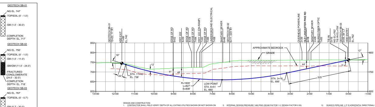
2. THE MINIMUM SEPARATION DISTANCE FROM EXISTING SUBSURFACE UTILITIES SHALL NOT BE LESS THAN 10 FEET AS MEASURED FROM THE OUTSIDE EDGE OF THE UTILITY TO OUTSIDE OF PROPOSED PIPELINE.
