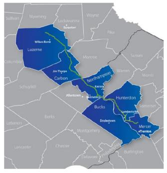
The proposed pipeline will extend more than 100 miles across two regions of the Pennsylvania Department of Environmental Protection (DEP). It is proposed to cross 3 counties in the Northeast Region, and 1 county in the Southeast Region. The proposed project involves the construction of pump stations, and includes avoidance of environmental or cultural resources and avoidance of surface features.
