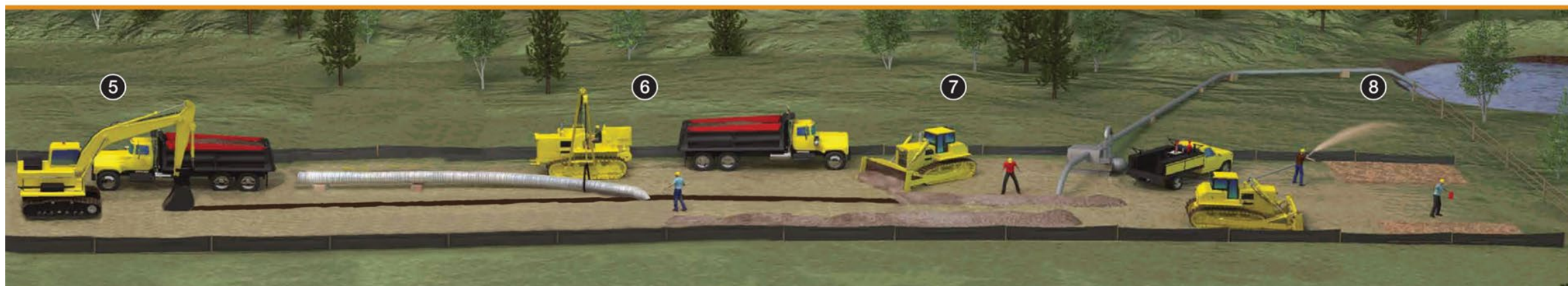
Figure A.2-1 Typical Pipeline Construction Sequence
