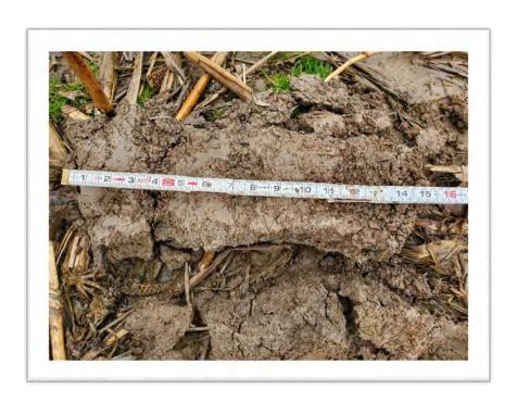
Photo 11: Soil Core of Wetland W2-PEM, Sampling Point DPK017 Showing F3
