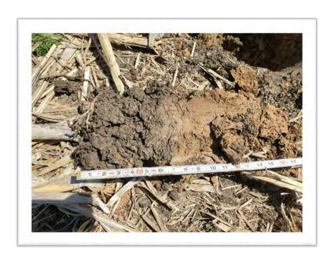
Photo 15: Soil Core of Wetland W6-PEM, Sampling Point DPK036 Showing F3
