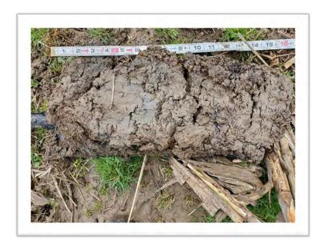
Photo 2: Soil Core, Wetland W1-PEM, Sampling Point DPK015 Showing Hydric F3
