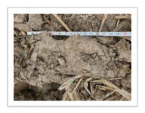
Photo 13: Soil Core of Wetland W4-PEM, Sampling Point DPK020 Showing F3
