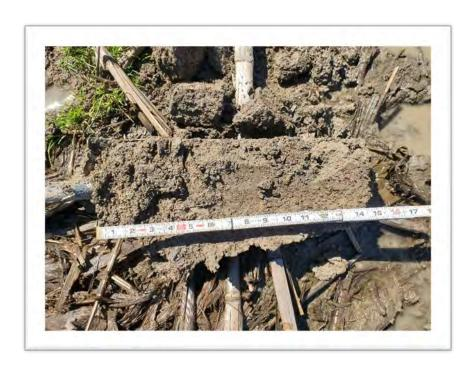
Photo 17: Soil Core of Wetland W9-PEM, Sampling Point DPK033 Showing F3
