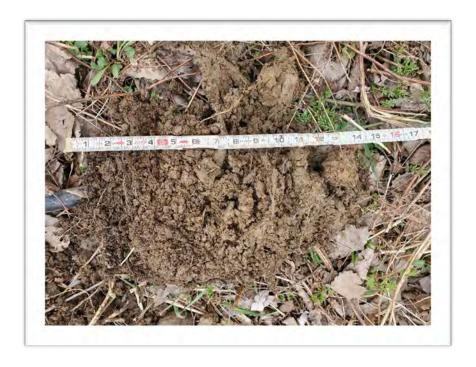
Photo 8: Soil Core of Wetland W1-PFO, Sampling Point DPK008, Showing F3
