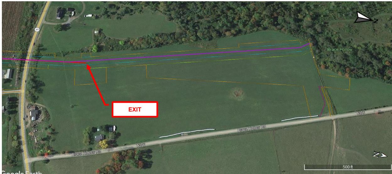
Figure 3. Proposed Pullback Workspace for Cowanesque River HDD
