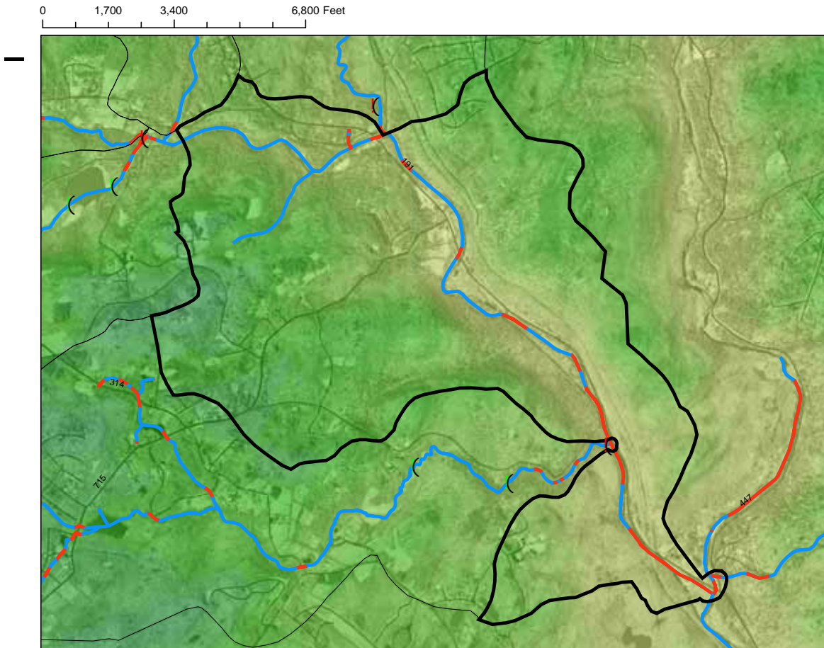
Figure 4 – Potential restoration sites in the Lower Paradise sub-watershed. Sites were identified by means of topographic map examination; stream proximity within 150 feet of roads, bridges and culverts; aerial photo examination and field verification.
