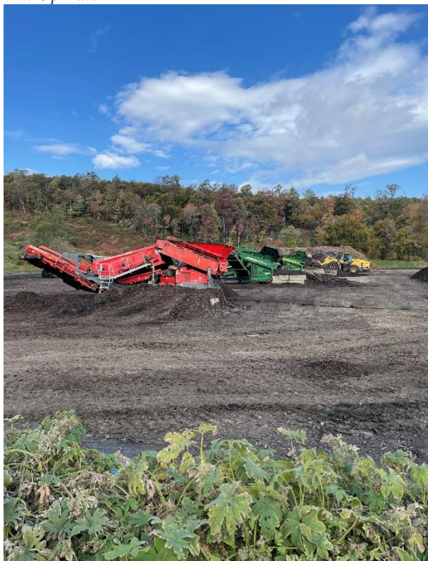
Screens Used for Removing Woodchips from Finished Product 20Oct2023
