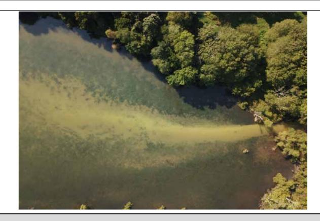
View of drilling fluid within stream S-H10 (UNT to Marsh Creek).
