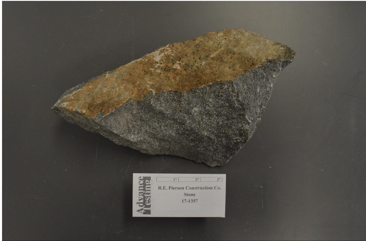
Specimen selected for petrographic analysis
