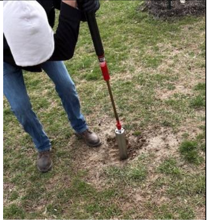
Subsurface soil collected with slam-bar/soil coring tool
