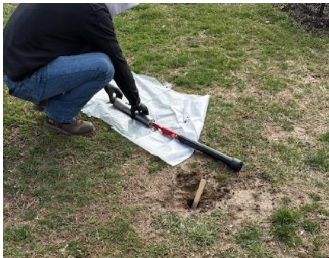
Soil core is recovered on clean plastic, to be placed in collection jar. Wood stick in hole used to ensure proper depth of core. 3/17/2025 @ 1627
