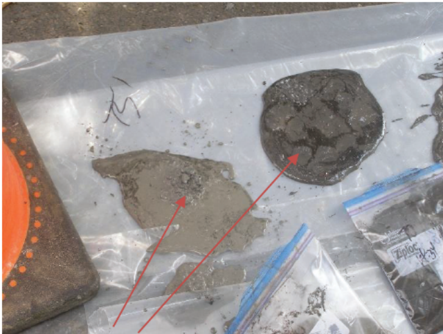
"Coal ash" in soil from MW-4D between 70-75 feet below asphalt 7-24-25 @ 14:36
