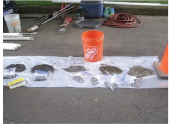
Soil samples from installation of monitoring well MW-4D 7-24-25 @ 14:17
