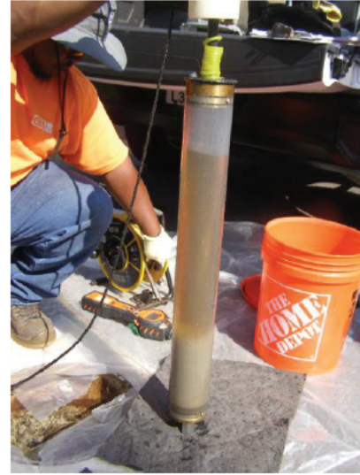
Mixture of LNAPL and emulsified LNAPL in skimmer when removed from recovery well RW-2 on Glenwood Drive 7-24-25 @ 9:48
