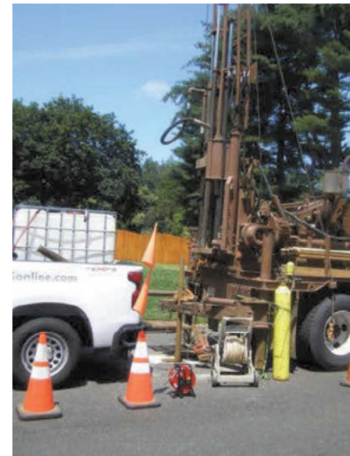
Packer testing set up at recovery well RW-2 6-23-25 @ 11:31
