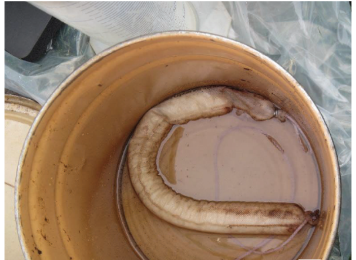
Absorbent sock removed during gauging of [redacted] potable well.
