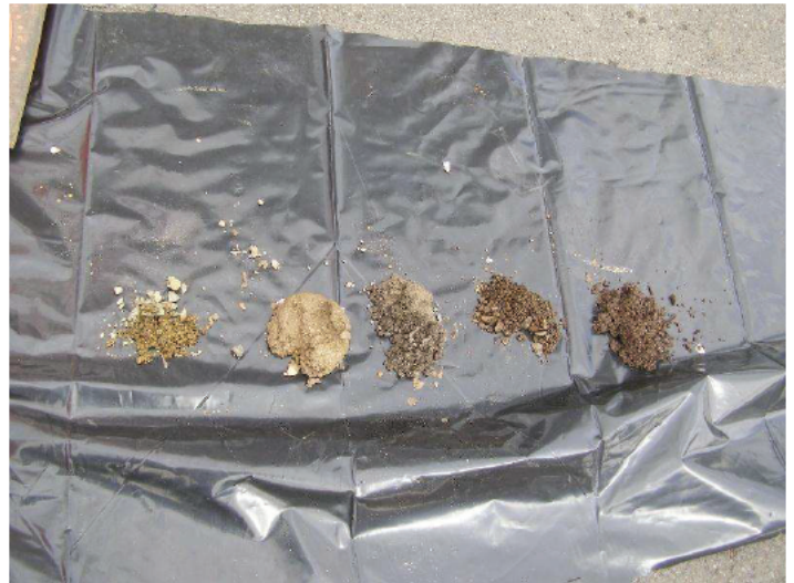
Photo 4: Soil and rock fragments collected during drilling Source: Olivia Budnovitch, 4/22/26
