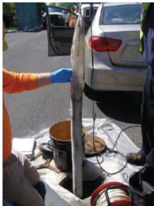
Removed sock from recovery well RW-3 4-27-26 @ 10:54
